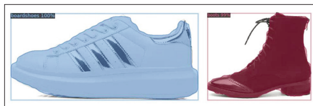
Fig. 4. The result of instance segmentation by removing shoes from the background of the image
